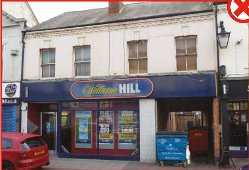
**POOR DESIGN.** The ground floor elevation of this building on Far Gosford Street has been totally removed by the modern shopfront which cuts across two historic properties. The individuality of the two properties has been lost and the ground floor shopfront design relates badly to the first floor above.
