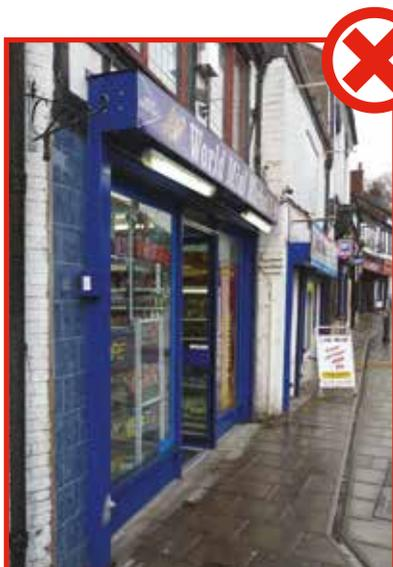
**POOR DESIGNS.** Externally fitted shutters like these are inappropriate in a Conservation Area or for a historic building.
