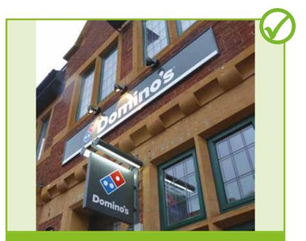
**GOOD DESIGN.** An example of a national chain adapting their house style to fit in with the Conservation Area requirements. A well-proportioned timber sign with a moulded edge, illuminated by discreet spot lights.
