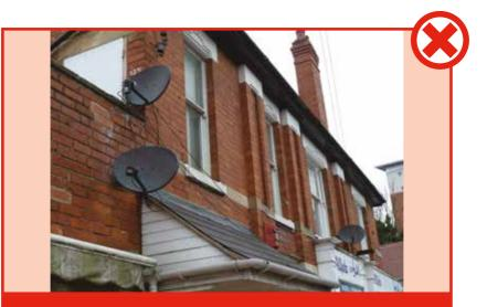
**POOR DESIGN.** Three poorly located satellite dishes on a single property, any redundant dishes should be removed and the rest should be relocated to the rear elevation away from the street.
