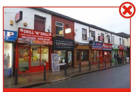
**POOR DESIGN.** Examples of mostly poor quality shopfronts in Far Gosford Street; external rollershutters, overly large internallyilluminated facia signs and projecting signs, poor quality replacement upvc windows of the first floor.
