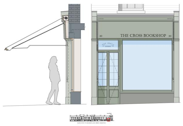
Figure 73. Front façade works, proposed new shopfront (typical).
