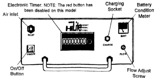
**FLOW ADJUST.** Below the level of the hole marked FLOW is a small screw. To adjust the flow use a small screwdriver, making sure the screwdriver end is located in the slot. To increase the flow turn clockwise. The span of this screw is around 5 turns. **DO NOT FORCE** the flow adjust screw, and Flow range by this adjuster is approximately 3-12 l/min. to free air.
