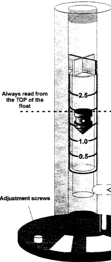
The SKC rotameter is supplied with an adapter and two pipe stub fittings which should be screwed into position as shown in the diagram opposite. This provides a method of connecting either a sampling head or flexible pipe to the rotameter.
