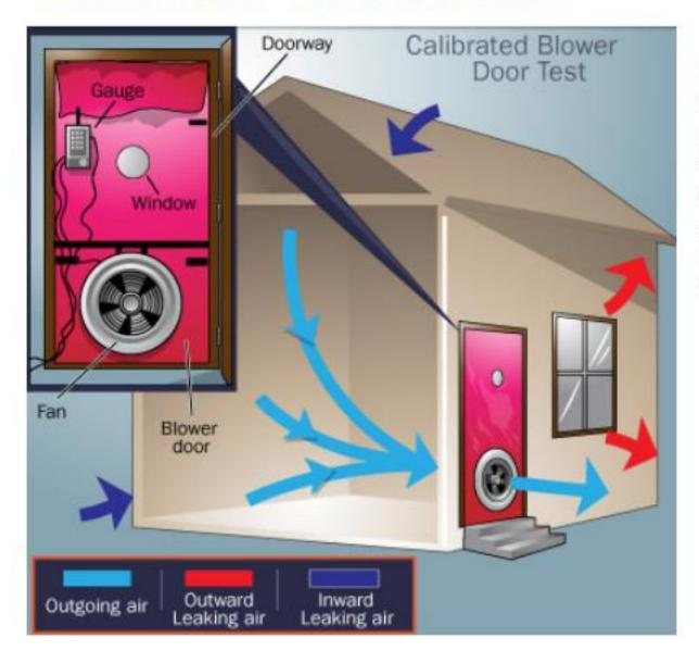
All of the air leakage paths occurring within a dwelling will have particular aerodynamic characteristics that are dependent upon the direction in which the air is flowing.
