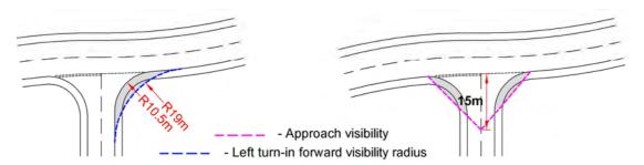
The approach visibility should be checked for local distributor and non-residential roads and connecting streets. It is measured 15m back from the give way line along the centreline of the side road. Drivers should be able to clearly see the layout of the junction on approach to the main road.
