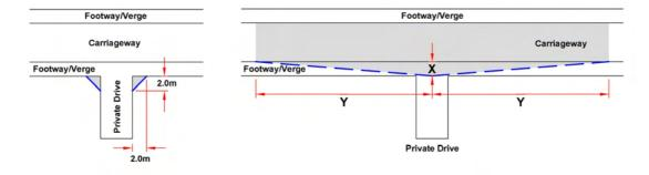
The **X** distance should be 2.0m for private drives and 2.4m for shared drives. The **Y** distance is the minimum forward visibility distance of the main road.
