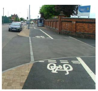
Cycle track with block paving buffer strip
