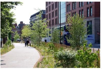
Grey to Green, Sheffield (left) and reed beds, Upton (above). Swales are used to retain rainwater and clean it of its pollutants via the stone, underlying soils and planting.
